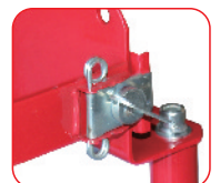
Rotate the knife at the opposite direction for lock tight
